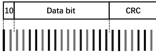
Fig. 5. Example of a MagCode Label. MagCode encodes data into evenly-spaced black and gray rectangular blocks. It uses their difference in magnetic field intensity to convey information. The first two bits are used to compare the similarity of intensity for “1” and “0”. The CRC is used by the label reader to verify the correctness of decoding. For illustration, 70% gray scale is used for the gray lines in this figure. We note that in real MagCode labels, the gray scale is close to or larger than 100%. As a result, the blocks can hardly be differentiated from their visual appearance.
